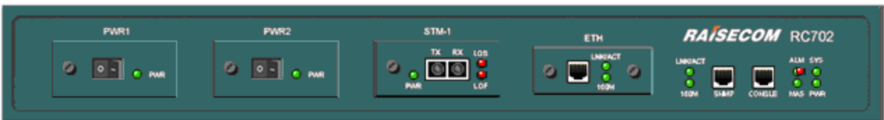
Figure 4-2 RC702 SDH fiber interface + Fast Ethernet copper interface front panel
